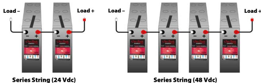
Batteries are placed in series (negative to positive) for additive voltages. Batteries in series are known as a "string". A string of two EnergyCell batteries has a nominal voltage of 24 Vdc and can be used for 24-volt loads. A string of four has a nominal voltage of 48 Vdc. Other voltages are possible. However, batteries in series do not have additive amp-hours. A single string of any voltage (as shown above) has the same amp-hours as a single battery.
